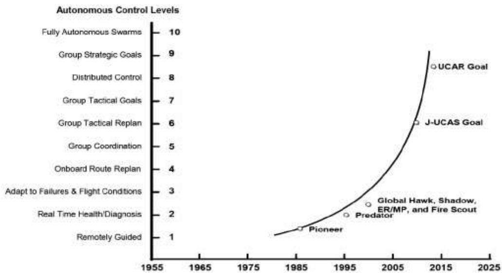
Fig. 13 – Gli Autonomous Control Level del AFRL<sup>69</sup>
