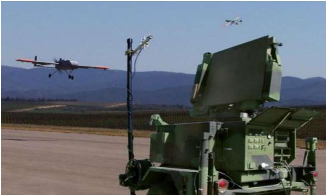
**Fig. 20 - Ground Based Sense and Avoid, RADAR-based**
